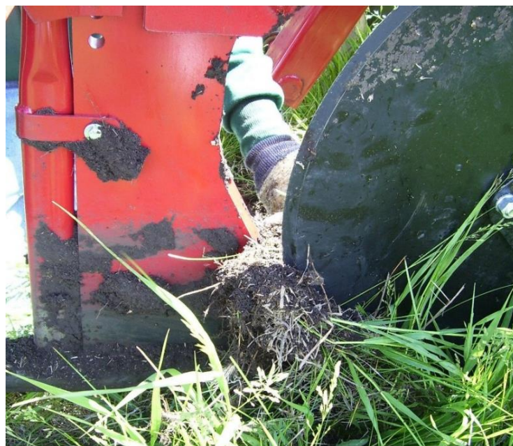
Figure 13: Roots catching on knife due to coulter blade set too shallow
