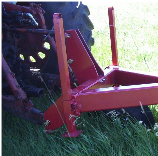
Figure 10: GA-800 Attachment to a Category 2 Three Point Hitch
