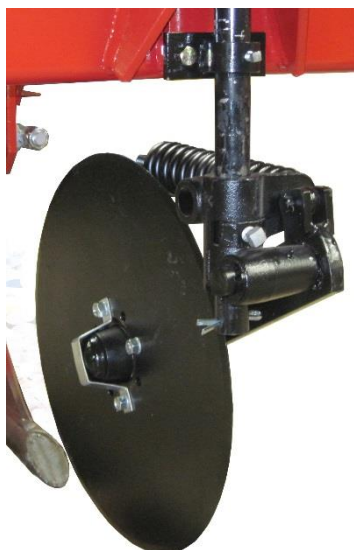
Figure 9: Completed Coultter Assembly
